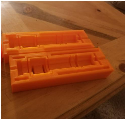
(a) 3D printed mount for  $^3\text{He}$  probe: top and bottom halves.
