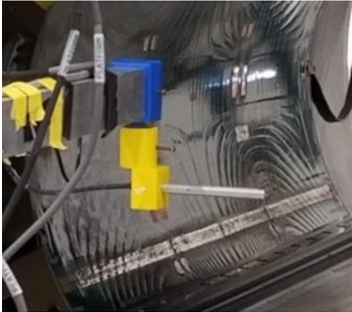
(a) UW NMR Probe mounted on 3D stage using one-sided mount.
