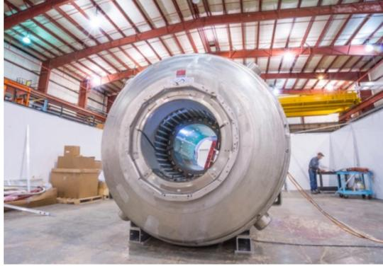
Figure 5.1: High field superconducting MRI magnet at Argonne National Lab.
