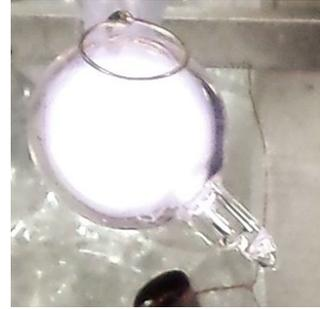
(b) Single  $^3\text{He}$  cell and stem after pull off. The loop of wire is one of the two coils connected to the transformer used to strike the discharge.
