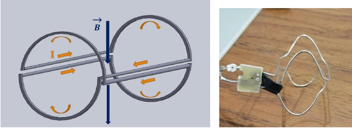
(a) Saddle coil drawing: current direction indicated with orange arrows, magnetic field direction in blue. (b) Photo of first saddle coil with tuning capacitors soldered on.
