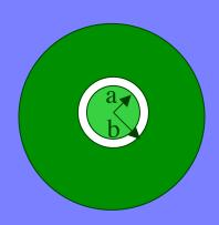
C/L =  $2\pi \Box_0 \Box / \ln(b/a) \sim a/t$ b=a+t a=10  $\mu$ m, t = 0.1  $\mu$ m C/L= 5.5 pF/mm
