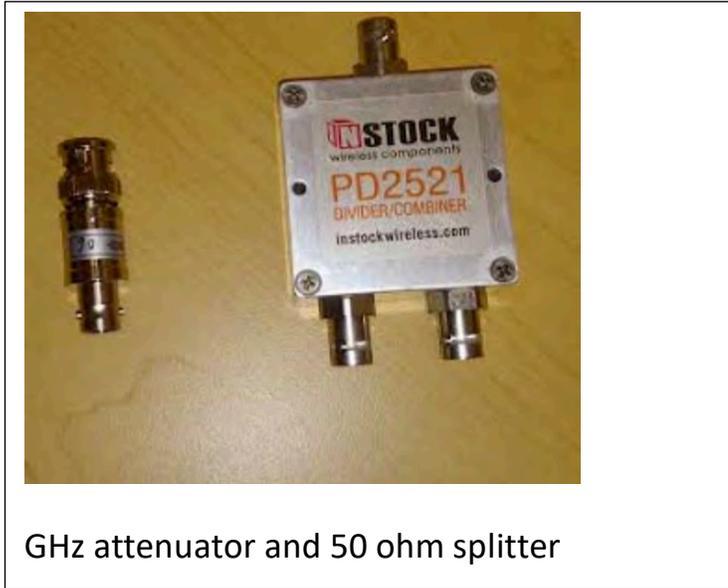
GHz attenuator and 50 ohm splitter
