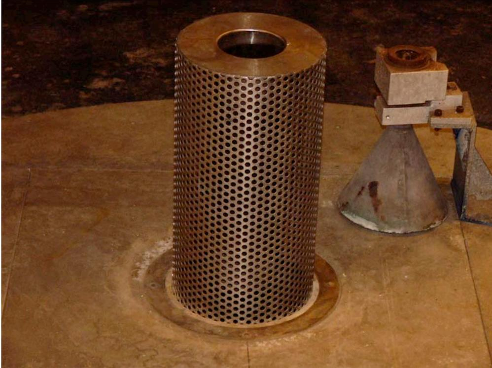
**Figure 3.16** The cover and the lid on the well of the gamma source
